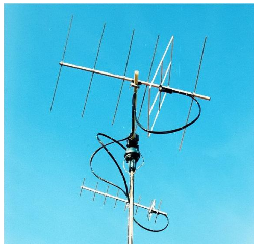
Figure 16 - Crossed yagi antenna in a fixed outdoor installation.
