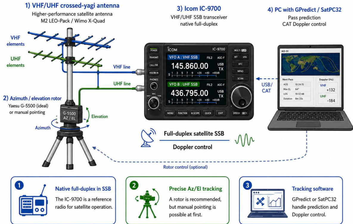
Figure 14 - SSB satellite station with IC-9700, Az/El rotator and PC.
