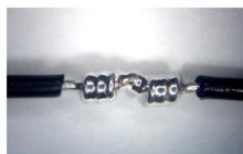
Figure 19-18. Soldered Western Union/Lineman Splice
